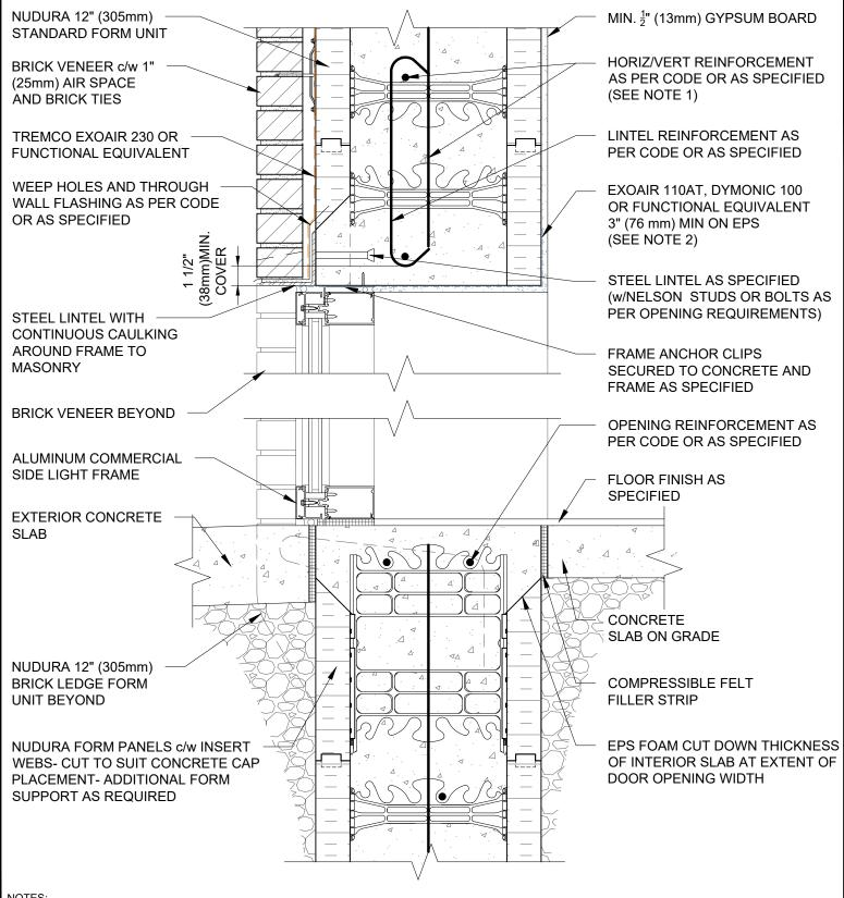
1) FOR OPTIMAL REINFORCEMENT PLACEMENT IN THE NUDURA FORM, SPACING OF HORIZONTAL REINFORCEMENT TO BE SPECIFIED AT 18" (457mm) O.C. AND VERTICAL REINFORCEMENT TO BE SPECIFIED AT MULTIPLES OF 8" (203mm) O.C. REFER TO NUDURA REINFORCEMENT PLACEMENT DETAILS. 2) AIR BARRIER/DRAINAGE FLASHINGS TO BE INSTALLED AROUND COMPLETE OPENING PERIMETER AS PER TREMCO/NUDURA APPLICATION INSTRUCTIONS OR AS DETAILED BY LOCAL APPLICABLE CODES (CODE GOVERNS).
